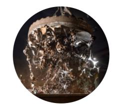
wire briquettes, which primarily consist of metal wire from end-of-life car tyres and cast iron shavings. These briquettes make a key contribution to the company's recycling efforts and support the goal of increasing the use of alternative scrap sources:
